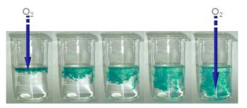
In order to avoid the formation of skin **ANTIGEL**<sup>®</sup> **KF / ANTIGEL**<sup>®</sup> **KF-D** are used. They interfere in the oxidation process and prevent the reaction of oxygen with the resin molecules.
